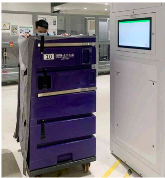
醫院被服從洗衣槽送到洗衣車的那一刻起，再送到污衣被服室，都可以透過無線射頻辨識技術進行密切監控 The hospital linen can be closely monitored with RFID, from the moment it is sent from linen chutes to laundry carts, to the soiled linen room
